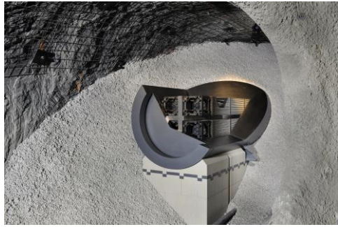
A 1:1 model of an emplacement drift for high-level waste is exhibited at the Mont Terri Rock Laboratory. Source: © Comet Photoshopping, Dieter Enz
