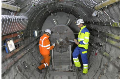
Research on safe disposal of radioactive waste is being carried out in the Mont Terri Rock Laboratory. The FE Experiment is a 1:1 demonstration experiment of an emplacement drift for high-level waste. Source: © Comet Photoshopping, Dieter Enz
