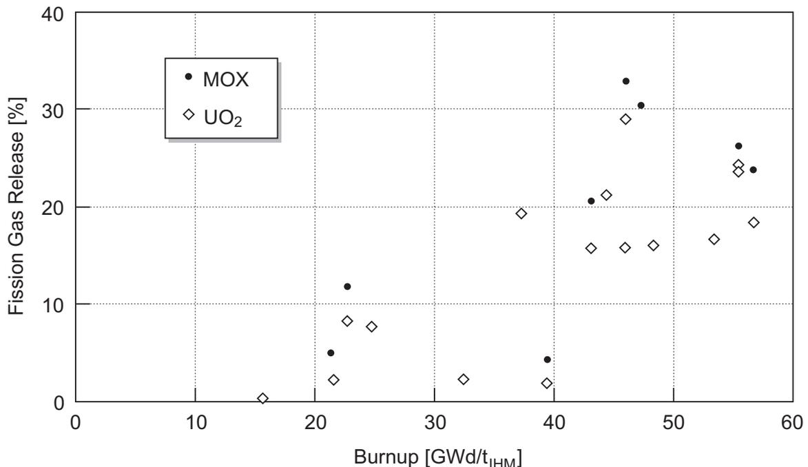
Figure 9: Fission gas release from BWR MOX and  $\text{UO}_2$  fuel (HAAS & LIPPENS 1997)
