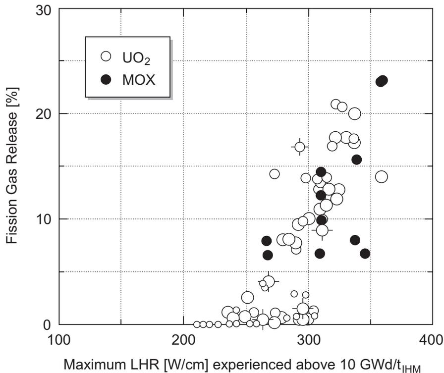
Figure 2: Fission gas release of BWR-MOX and  $\text{UO}_2$  fuels as a function of the linear heat rating (in  $\text{W/cm}$ ), from KAMIMURA (1992).
