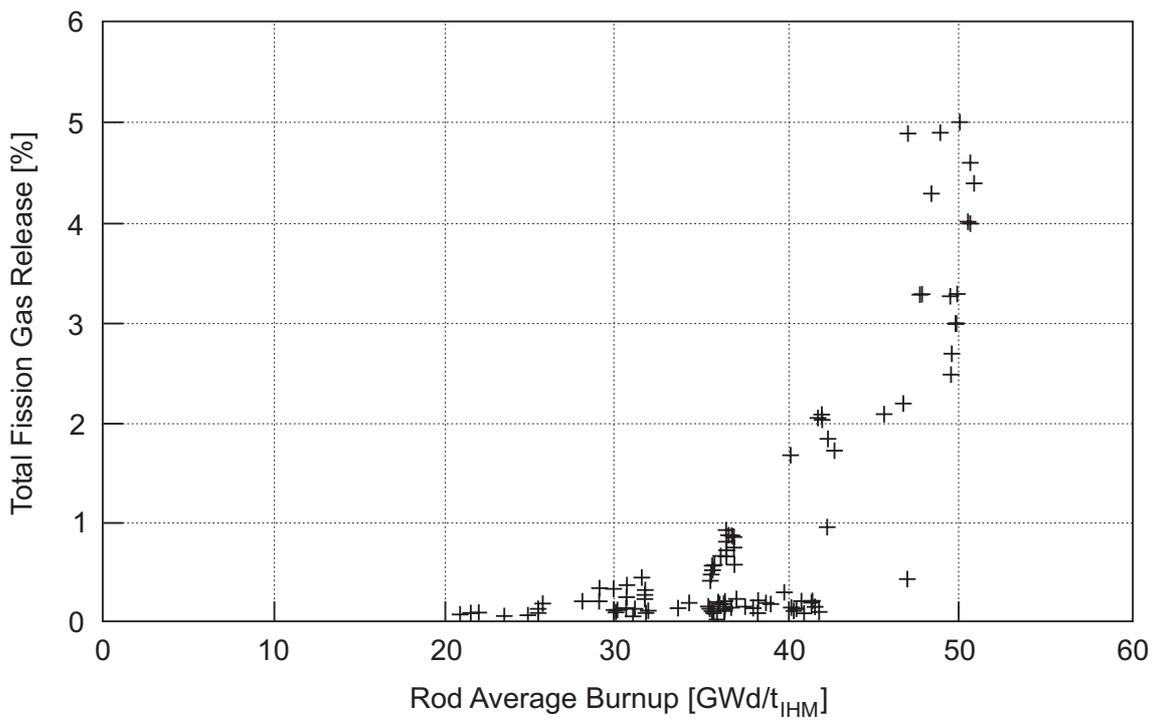
Figure 5: Fission gas release of BWR fuel as a function of average rod burnup (SCHRIRE et al. 1997)
