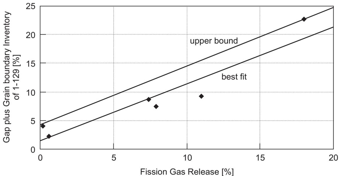
Figure 11: Gap plus grain boundary release of I-129 vs. fission gas release (data from Table 2)
