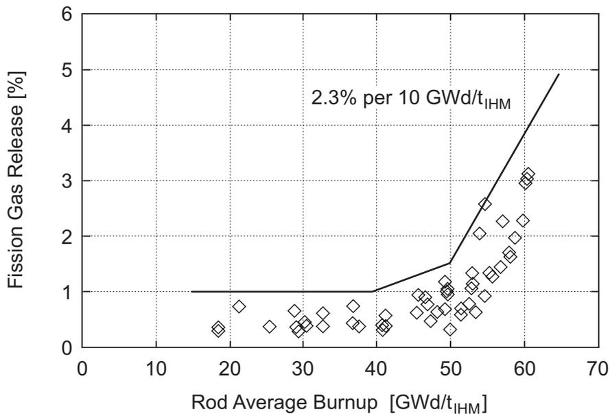
Figure 3: Fission gas release from PWR fuel as a function of burnup (VESTERLUND & CORSETTI 1994). The line represents the bounding values of all the data.
