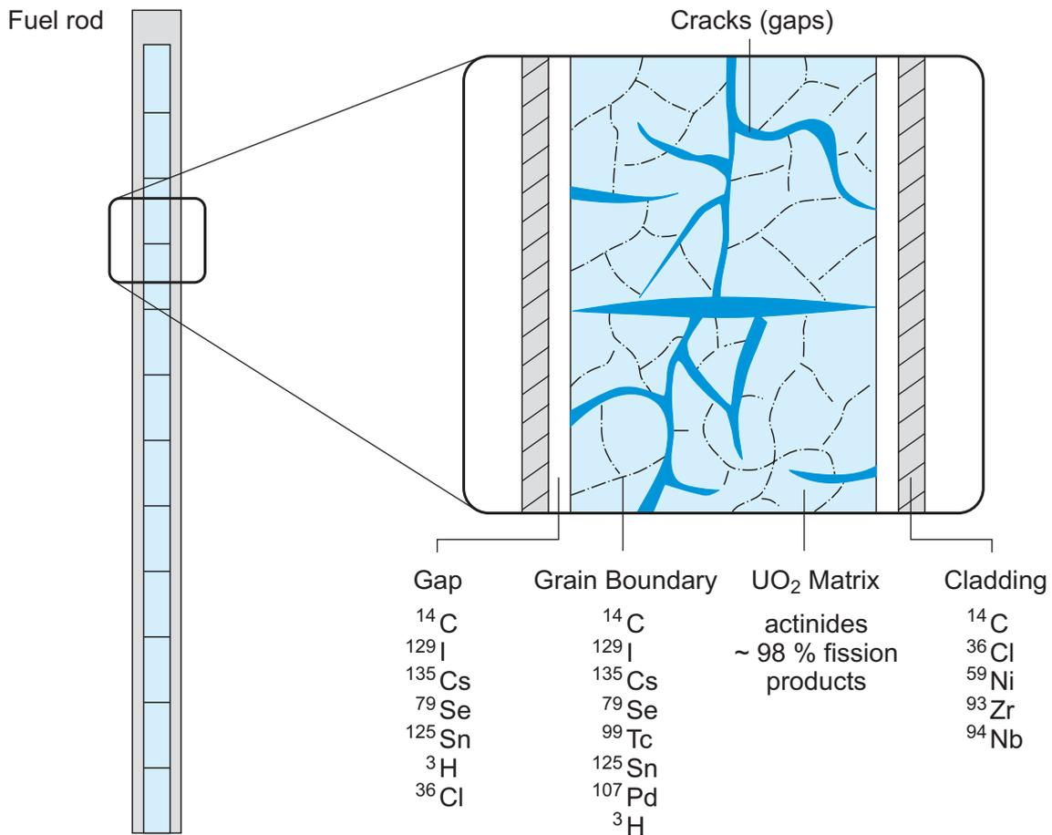
Figure 1: Conceptual distribution of some fission and activation products within a spent fuel element
