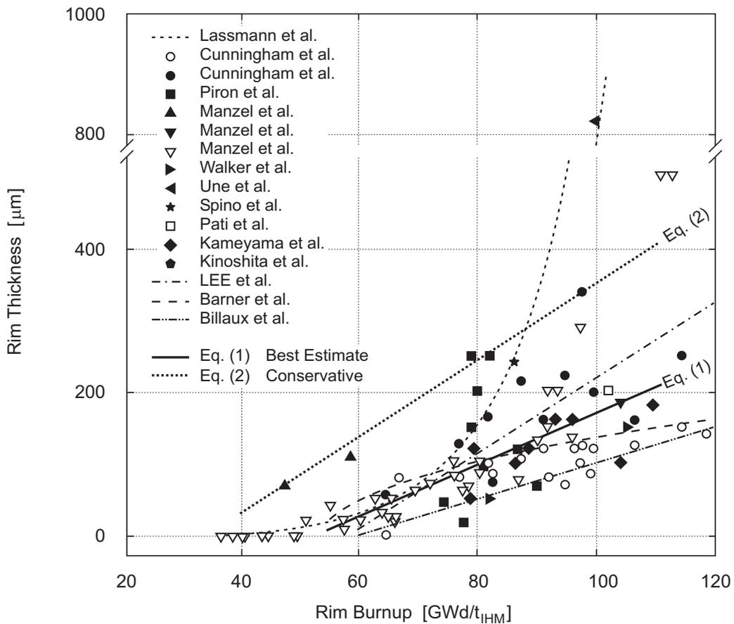
Figure 7: Rim width in  $\mu\text{m}$  as a function of burnup ( $\text{GWd/tU}$ ), from KOO et al. (2001). Equation 1 represent a best fit of the data, while Equation 2 is a conservative or bounding expression that encompasses almost all the data. The references and equations referred to are in the paper by KOO et al. (2001).
