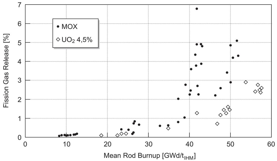
Figure 6: Fission gas release for French LWR UO<sub>2</sub> and MOX fuel as a function of burnup (GUERIN et al. 1999)
