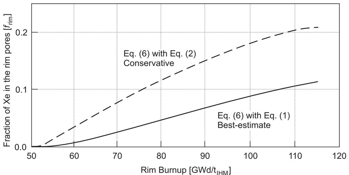
Figure 8: Fraction of total Xe inventory trapped in rim pores as a function of rim burnup, from KOO et al. (2001). Equations 1, 2 and 6 are given in the original paper.
