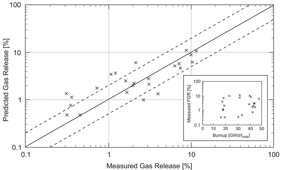
Figure 10: Predicted vs. measured fission gas release for MOX fuel (from GATES et al. 1998)
