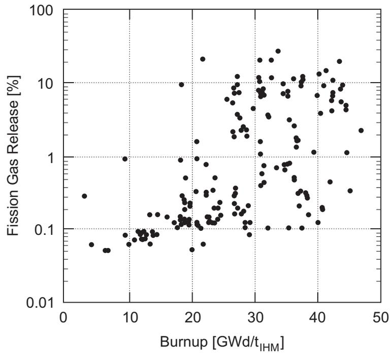
Figure 4: Fission gas release as a function of burnup for ABB BWR fuels (HALLSTADIUS & GRAPENGIESSER 1990)
