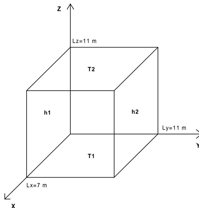
**Figure 6.4:** Schematic representation of the three-dimensional flow domain used in the model.
