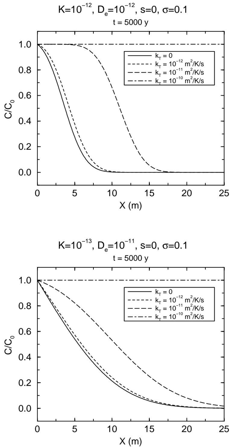
**Figure 5.2:** Relative concentration vs. distance at  $t = 5000$  y, for (a) hydraulic conductivity  $K$  equal to  $10^{-12}$  m/s, and (b) effective diffusion coefficient  $D_e$  equal to  $10^{-11}$  m<sup>2</sup>/s. The different curves in both plots correspond to different values of the thermo-osmotic permeability  $k_T$ .
