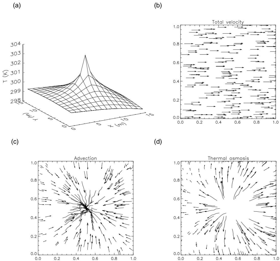
**Figure 6.3:** Results for case 2 ( $T_1 = 299.22$  K,  $T_2 = 298.08$  K). (a) Temperature, (b) total specific discharge, (c) advective component of the total specific discharge, and (d) thermal-osmotic component of the total specific discharge. Notice how the advective component of flow cancels the thermal-osmotic component, and there is no net effect of thermal osmosis arising from the presence of a heat source in the interior of the domain on the flow field.
