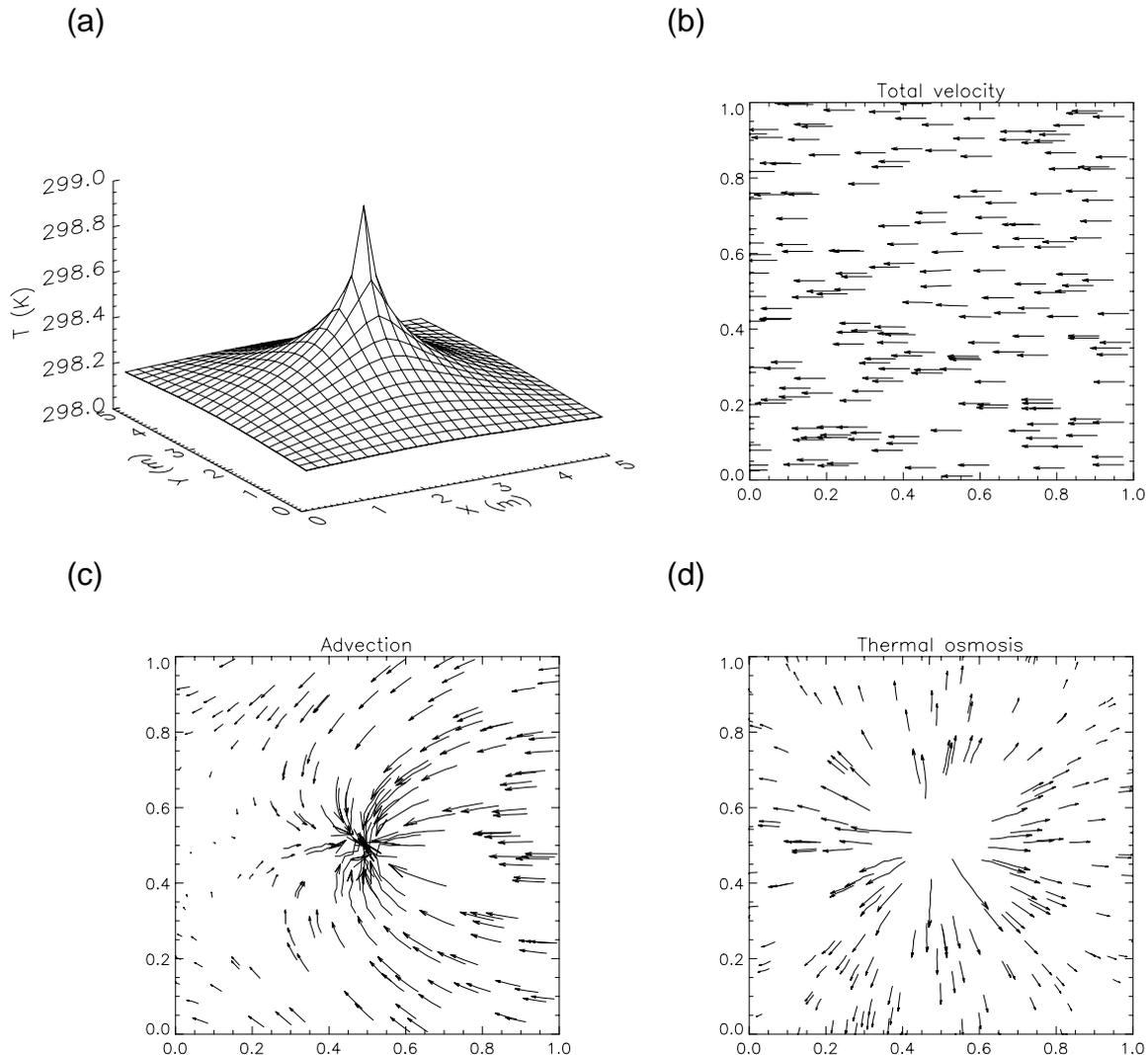
**Figure 6.11:** Results for the two-dimensional simulation with temperature-dependent density and viscosity. (a) Temperature, (b) total flow velocity, (c) advective component of the of the total velocity, and (d) thermal-osmotic component of the total velocity. Notice how the advective component of flow cancels the thermal-osmotic component, and there is no net effect of thermal osmosis on the flow field.
