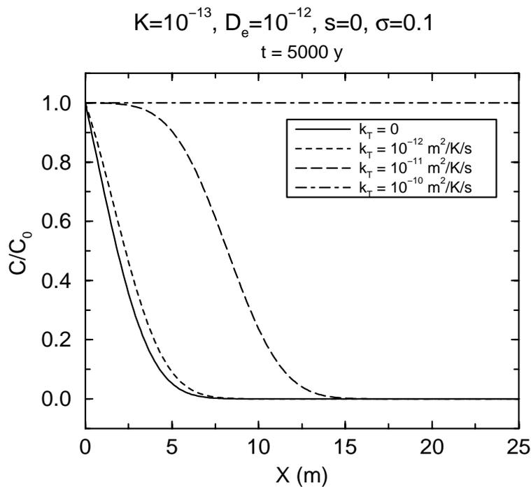
**Figure 5.1:** Relative concentration vs. distance at  $t = 5000$  y. The different curves correspond to different values of the thermo-osmotic permeability  $k_T$ . Thermal osmosis will only have a significant effect if  $k_T > 10^{-12}$  m<sup>2</sup>/K/s.
