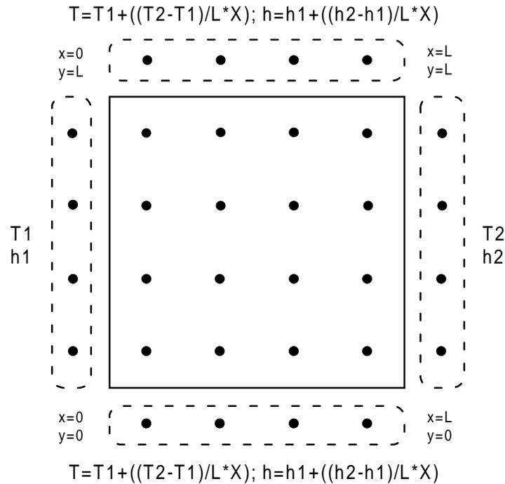
**Figure 6.1:** Schematic diagram showing the geometry and boundary conditions of the flow domain used in the model. The flow domain is enclosed by a thick solid line. External nodes, where the boundary conditions are defined, are enclosed by dashed lines.
