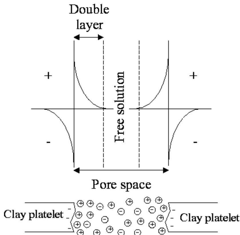
Figure 1.1: Electrical double layer in a clay pore (after MARINE & FRITZ, 1981)
