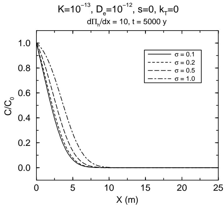
**Figure 5.4:** Relative concentration vs. distance at  $t = 5000$  y, for the case with an osmotic pressure head gradient ( $\partial\Pi_h/\partial x$ ) equal to 10. (a) Results for different values of the thermo-osmotic permeability  $k_T$ . (b) Results for different values of the osmotic efficiency  $\sigma$ , with  $k_T = 0$ .
