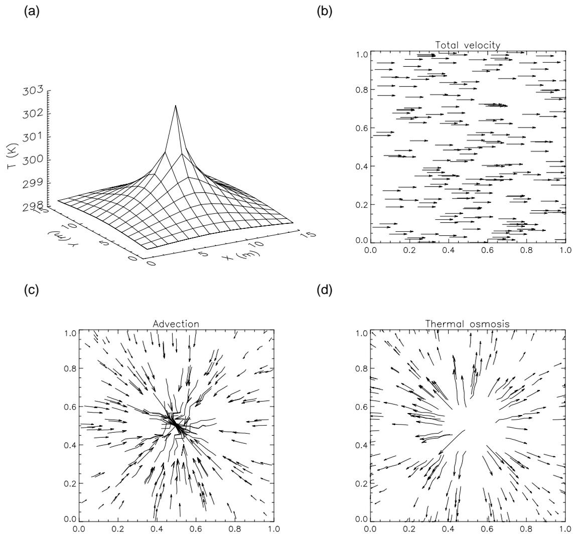
**Figure 6.2:** Results for case 1 ( $T_1 = T_2 = 298.15$  K). (a) Temperature, (b) total specific discharge, (c) advective component of the total specific discharge, and (d) thermal-osmotic component of the total specific discharge. Notice how the advective component of flow cancels the thermal-osmotic component, and there is no net effect of thermal osmosis on the flow field.
