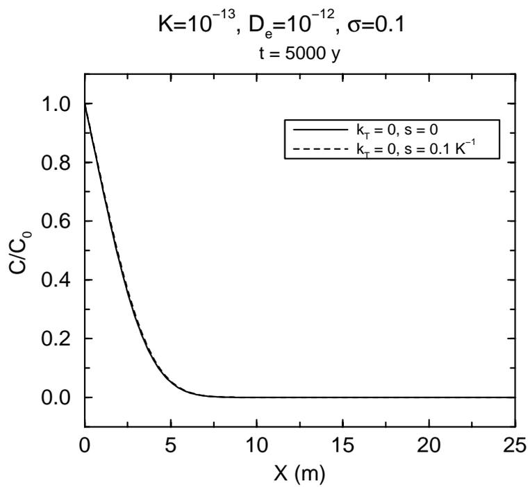
**Figure 5.3:** Relative concentration vs. distance at  $t = 5000 \text{ y}$ , for two different values of the Soret coefficient ( $s = 0$  and  $s = 0.1 \text{ K}^{-1}$ ).
