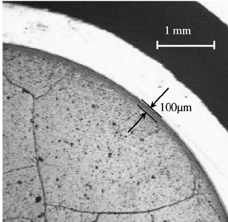
Fig. 5: Photograph of spent fuel showing the high burnup rim region adjacent to the cladding (Fors et al. 2009)
