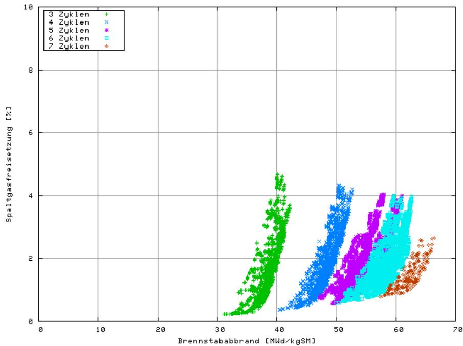
Fig. 2: FGR at end of cycle (EOC) for UO<sub>2</sub> fuel assemblies at KKB (AREVA 2012)
