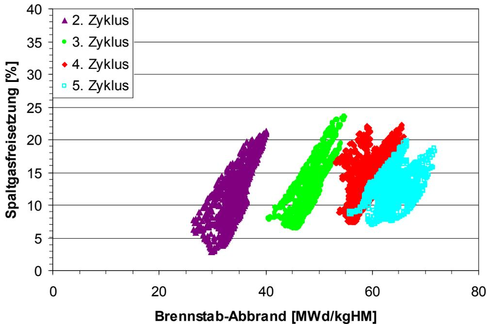
Fig. 3: EOC FGR of  $\text{UO}_2$  fuel assemblies for KKG 5 region core (AREVA 2010)
