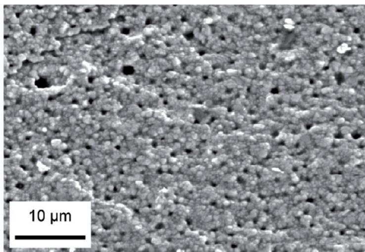
Fig. 6: Scanning electron microscopy micrograph of the high burnup rim region with a local burnup of 75 MWd/kgHM (Rondinella and Wiss 2010).
