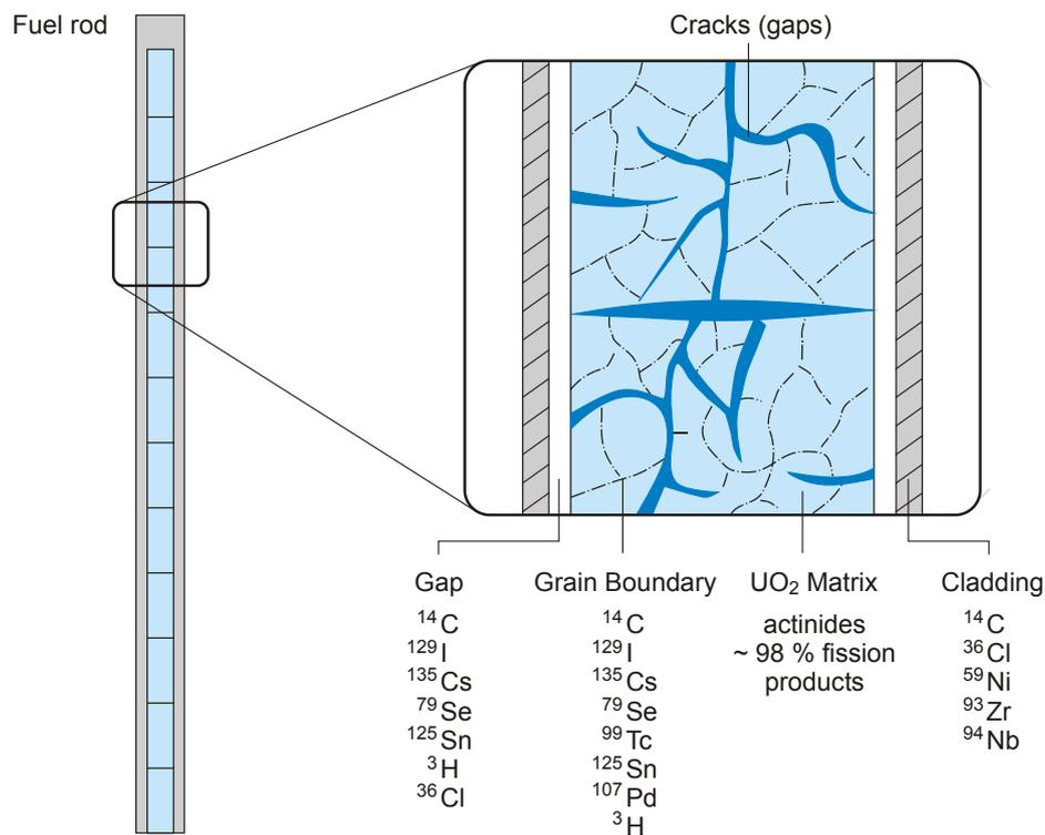
Fig. 1: Conceptual distribution of radionuclides in a spent fuel rod, based on Johnson and Tait (1997).
