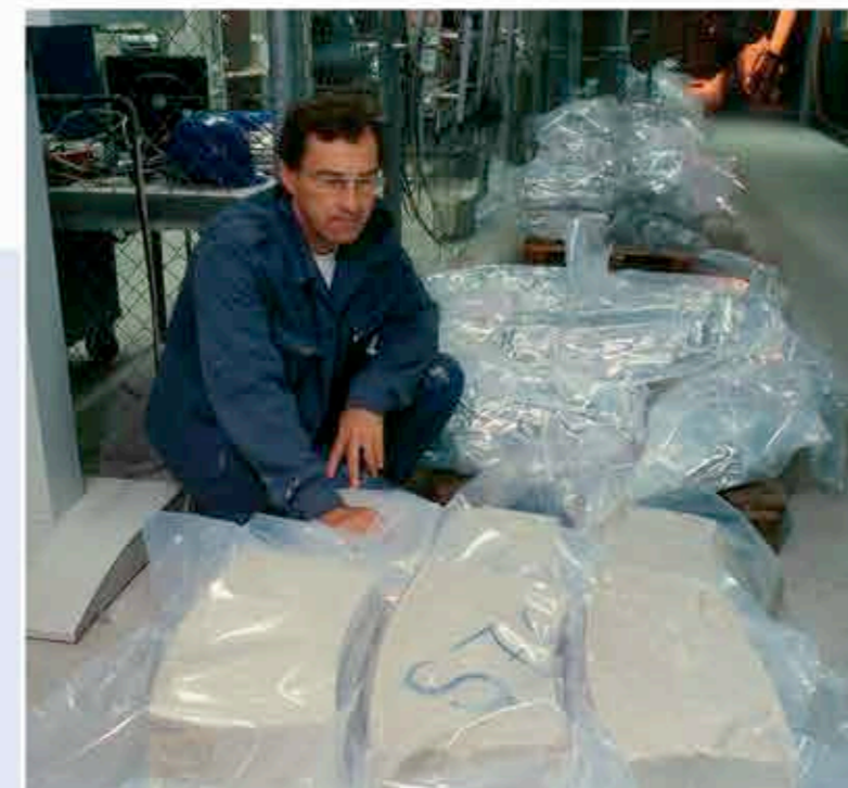
As part of the FEBEX experiment being carried out in a tunnel at the Grimsel Test Site, the safety barrier system for a geological repository for high-level waste is being investigated. After six years, the system was partly excavated and more than 1000 material samples were collected. The samples are being analysed in the laboratories of the 23 partners in the FEBEX project. The photograph shows the bentonite blocks used as a tunnel backfill.
