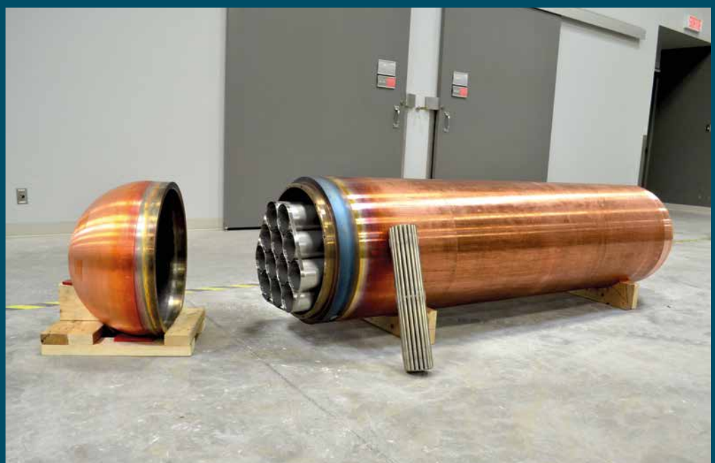
Prototype of a steel canister with a copper coating
