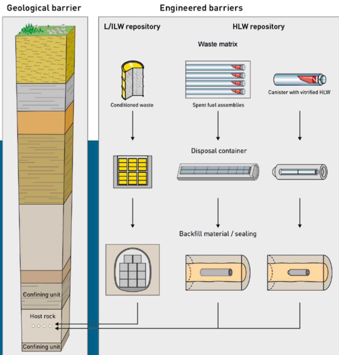
Multiple safety barriers provide containment of the radioactive substances in a deep geological repository and largely prevent release to the human environment. The geological barrier plays a decisive role in this respect.
